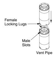
Figure 23 - Vent Pipe Connections
